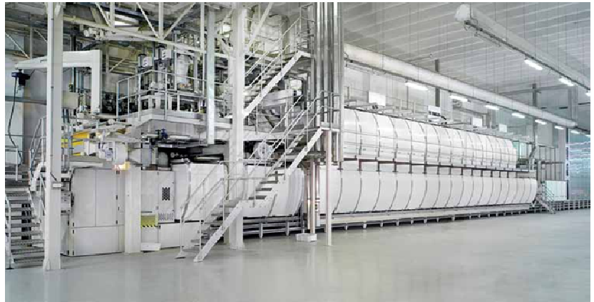
Pasta dryers are modular designed and contain 4 to 10 climate zones
