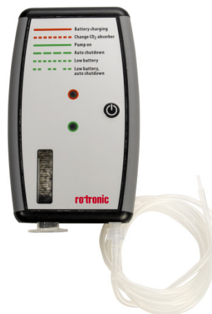
CP11 handheld device with the O-calibration unit
