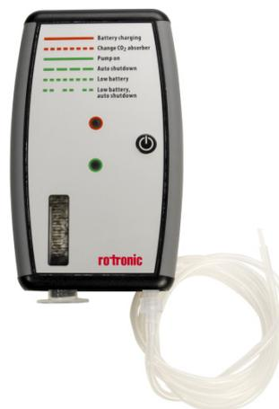
CL11 data logger with the 0-calibration unit
